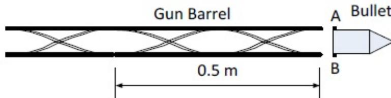
Helical slots are such that one turn of helix is completed over a distance of 0.5 m. If velocity of bullet when it exits the barrel is 20 m/s, its spinning speed in rad/s is \_\_\_\_\_
