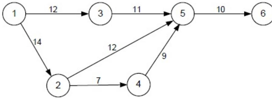
The minimum time (in days) for completion of the project is \_\_\_\_\_
