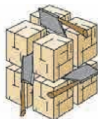
D) Galena has three sets of cleavage that form two 90^\circ angles (cubic cleavage)
