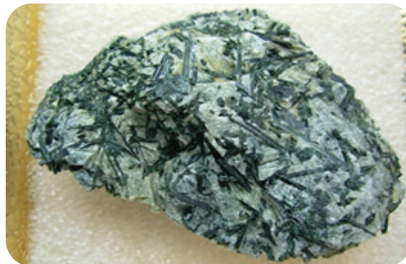
Fig. 5.24 : Acicular form in green coloured needles of Actinolite
