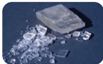
E) Calcite has three sets of cleavage - 105^\circ in one plane and 75^\circ in another
