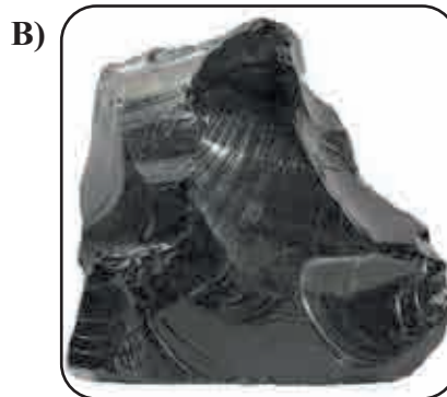
Fig. 5.41 : A) Conchoidal, B) Subconchoidal fracture
