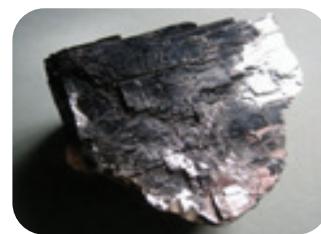
D) Galena has three sets of cleavage that form two 90^\circ angles (cubic cleavage)
