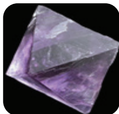
F) Fluorite has four sets of cleavage (octahedral cleavage)
