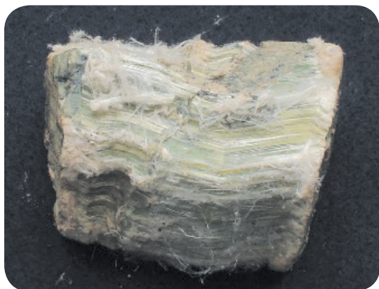
Fig. 5.44 : Splintery fracture in Serpentine
