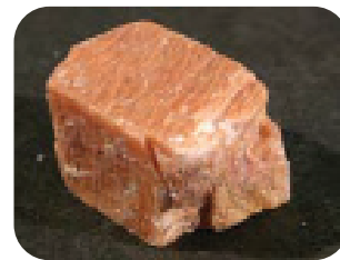
B) Orthoclase and plagioclase feldspars exhibit two sets of cleavage at approximately 90^\circ from each other.
