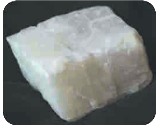
Fig. 5.19 : Subvitreous lustre in Calcite
