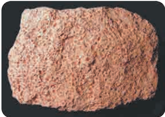
Fig. 5.35 : Oolitic form in Bauxite
