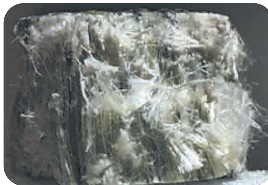
Fig. 5.26 : Fibrous form in Asbestos (Serpentine)
