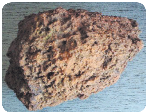
Fig. 5.42 : Earthy fracture in Limonite
