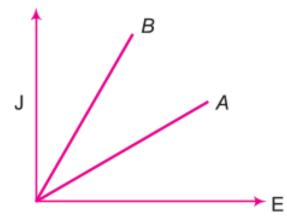
Let  $\rho A$  the resistivity of the standard resistance A and  $\rho_B$  is the resistivity of the connective wire, i.e.,  $\rho_B < \rho_A$ . So the graph of J vs E can be given as shown alongside.
