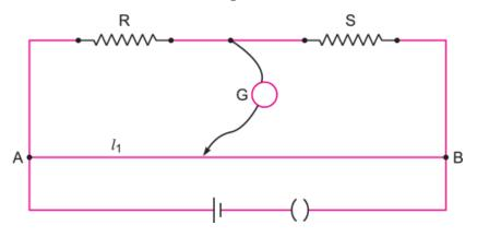
An unknown resistance X is now connected in parallel to the resistance S and the balance point is found at a distance  $I_2$ . Obtain a formula for X in terms of  $I_1$ ,  $I_2$  and S.
