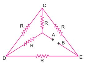
(ii) Also calculate the current through CD and ACB if a 10 V dc source is connected between points A and B and the value of R =  $2\Omega$ .
