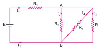
**Ans.** Given  $R_1 = 4\Omega$ ,  $R_2 = R_3 = 15\Omega$ ,  $R_4 = 30\Omega$ , E = 10 V.
