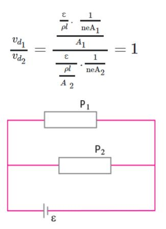
Q. 6. Two heating elements of resistance  $R_1$  and  $R_2$  when operated at a constant supply of voltage, V, consume powers  $P_1$  and  $P_2$  respectively. Deduce the expressions for the power of their combination when they are, in turn, connected in
