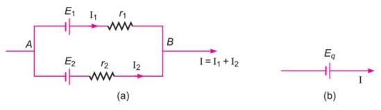
Let I1 and I2 be the currents leaving the positive, terminals of the cells, and at the point B
