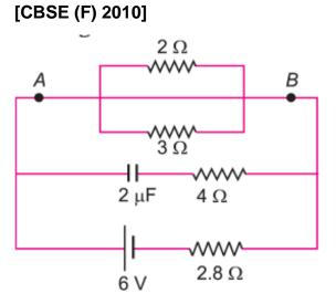
**Ans.** In steady state there is no current in capacitor branch, so equivalent circuit is shown in fig.
