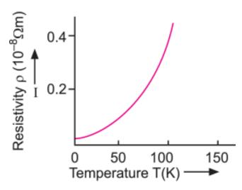
Resistivity  $\rho_T$  of metallic conductor as a function of temperature T
