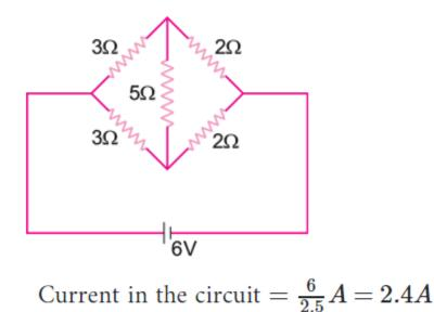
**Kirchhoff's Loop Law:** The algebraic sum of potential differences of different circuit elements of a closed circuit (or mesh) is zero. This law is based on law of conservation of energy.
