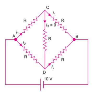
(i) The equivalent circuit is shown in fig. It is a balanced Wheatstone bridge. So, the resistance connected between C and D is ineffective.
