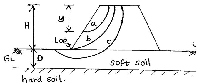
For base failure,  $D_F > 1$  (when there is soft soil)
