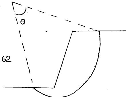
$$F_{QS} = \frac{C_L R}{w \bar{x}} = \frac{27 \times 30.62 \times 14.5}{1980 \times 3.75} = \underline{1.61}$$
