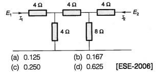
$\mathbf{Q.27}$  The currents  $I_1$  and  $I_2$  at the output of 2-port network can be written as
