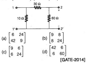
Q.42 A 2-port network is shown in figure. The parameter  $h_{21}$  for this network can be given by
