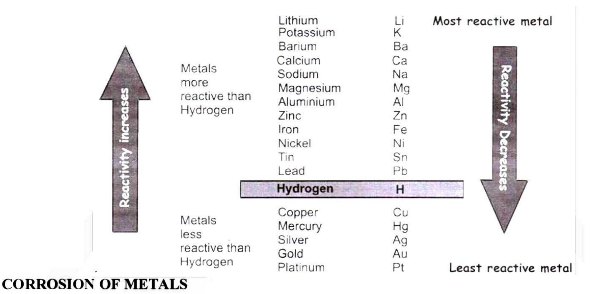
Corrosion is a process of deterioration of metal as a result of its reaction with air or water (present in environment) surrounding it.
