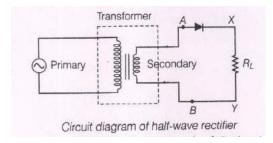
Now, the working, during half cycle of the input AC, then the p-n junction is forward biased. And the resistance in p-n junction becomes very low and diode works, therefore, current flows.
