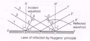
Let us suppose c is the speed of light, t is the time taken by the light to go from B to C or A to D or E to Go through F, then
