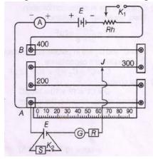
For the determining the resistance of cell in which the plug  $K_2$  is kept out and the jockey J is moved on the potentiometer
