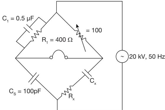
$$\text{Power factor} = \frac{R_x}{Z_x} = \omega R_x C_V = \omega R_1 C_1$$
