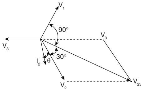
Phase difference between  $V_1$  and  $I_2$  is
