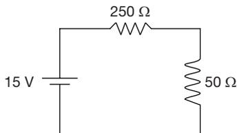
$$\text{Measured value of current} = \frac{15}{300} = 50\text{mA}$$
