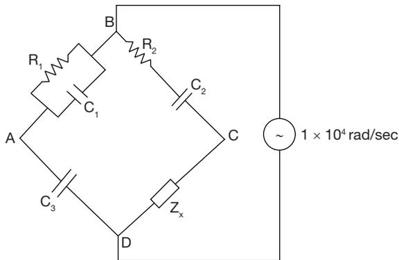
$$Z_x = \left\{ \frac{\omega^2 C_1 C_2 R_1 R_2 - 1}{\omega^2 R_1 C_2 C_3} \right\} - j \left\{ \frac{R_2 C_2 + R_1 C_1}{\omega R_1 C_2 C_3} \right\}$$
