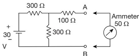
It is desired to measure the value of current in the 100 Ω resistor as shown in figure, by connecting a 50 Ω ammeter, the percentage error in measurement will be
