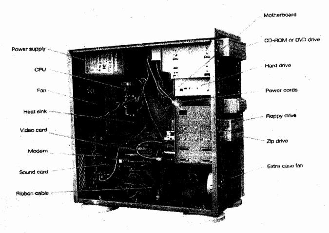
**Motherboard** - The motherboard is the main circuit board of a microcomputer. It is also known as the mainboard or system board.
