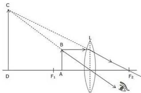
The object is placed between focal point  $F_1$  and convex lens and its image is formed at the same side of the lens which is enlarged.
