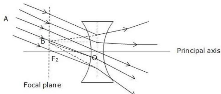
**Refraction of an oblique parallel beam by a concave lens**
