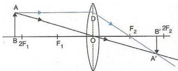
Here the candle is AB and its real and inverted image is formed between  $F_2$  and  $2F_2$ .
