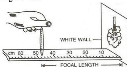
By moving the convex lens to and fro along the scale, focus a distant object on wall. The image which forms on the wall is very near to the focus of the lens and the distance of the lens from the image is read directly by the metre scale. This gives the approximate focal length of the lens.
