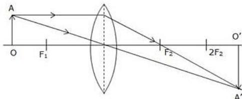
(b) The position of the images will be more than twice the focal length of lens.
