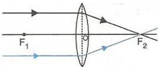
While using the convex lens as burning glass, the rays of light from the sun (at infinity) are brought to focus on a piece of paper kept at the second focal plane of the lens. Due to sufficient heat of the sun rays, the paper burns. Hence this lens is termed as 'burning glass'.
