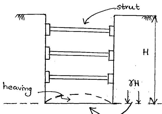
$$\text{FOS} = \frac{C N_c}{\gamma H} = \frac{20 \times 7}{20 \times 5} = \underline{\underline{1.4}}$$
