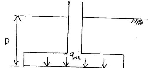
$$q_u = \gamma D \left( \frac{1 + \sin \phi}{1 - \sin \phi} \right)^2$$
