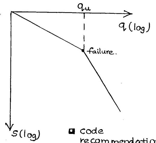
$$\text{Safe bearing capacity}, q_s = \frac{q_u}{F}$$
