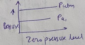
★ Gauge and vacuum may be (+ve) and (-ve) but atmospheric absolute pressure always (+ve) (Real Pressure)
