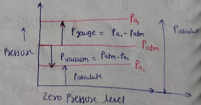
① Atmospheric Pressure → It is the pressure exerted by environmental mass
