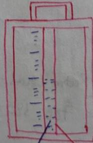
$\phi$  dia sufficiently large to neglect capillary effect
