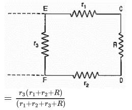
This value should be equal to R, so that by the repeated operation of this type will be left with only one square which will be the left extreme one and it will have a value R.
