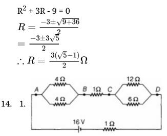
In circuit AB, 2 resistors of resistance  $4\Omega$  and  $4\Omega$  are connected in parallel combination.
