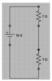
In the circuit , 2 resistors of resistance  $7\Omega$  and  $1\Omega$  are connected in series combination.
