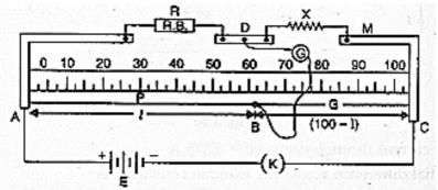
In the figure X is unknown resistor and R.B is resistance box. After inserting the key k, jockey is moved on wire AC till galvanometer shows no deflection (point B). If k is the resistance per unit length of wire AC.
