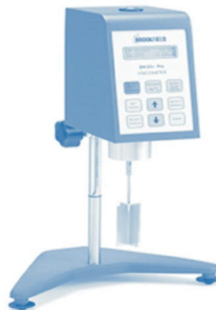
Fig.1.2. Viscometer for determination of viscosity of milk
