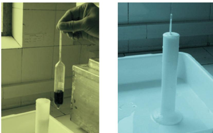
Fig.1.3. Determination of specific gravity of milk by ISI lactometer
