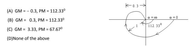
**Q.4** The open loop transfer function of a unity feedback control system is given as  $G(s) = \frac{1}{s(1+sT_1)(1+sT_2)}$ The phase crossover frequency and the gain margin are, respectively.
