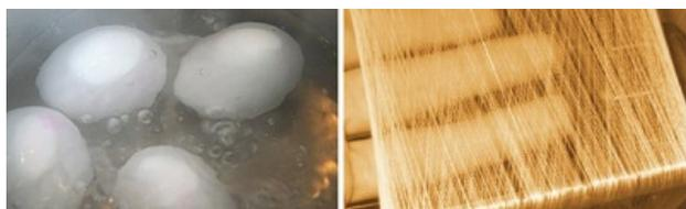
**Fig.** Boiling cocoon (left) and reeling of silk (right)
