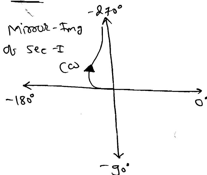
$\Rightarrow$  Sec-III is a mirror-image of Sec-I, about the Real axis but the direction is continuous.
