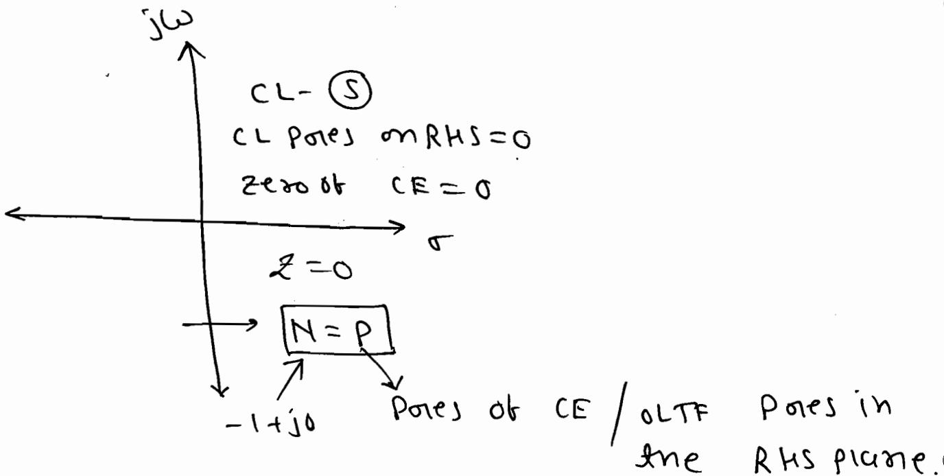
$\Rightarrow$  The Close-loop pole is nothing but, zeros of CE which must be zero, in the right of S-plane that means
