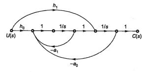
Assuming,  $h_1 = b_1$  and  $h_0 = b_0 - b_1 a_1$ , the inputoutput transfer function,  $G(s) = \frac{C(s)}{U(s)}$  of the system is given by
