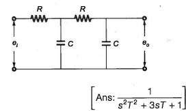
The transfer function of a low-pass RC network
