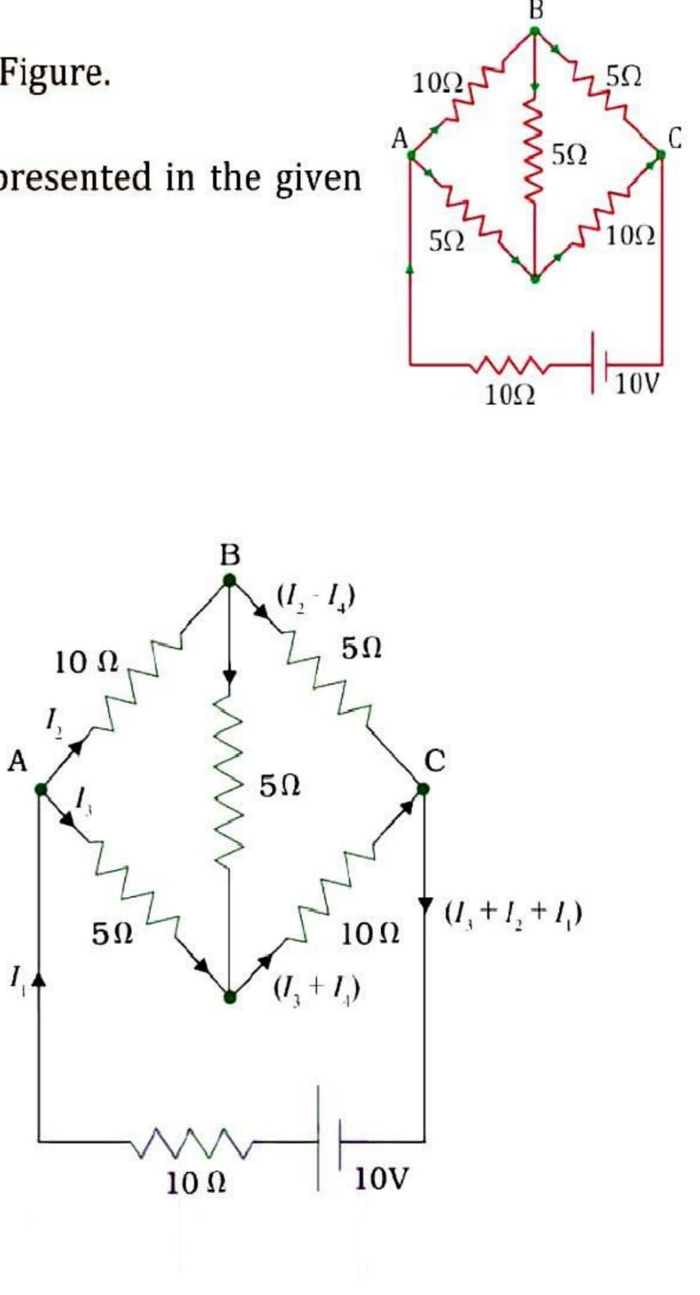
I<sub>2</sub> = Current flowing through branch AB  $I_3$  = Current flowing through branch AD I<sub>2</sub> – I<sub>4</sub> = Current flowing through branch BC I<sub>3</sub> + I<sub>4</sub> = Current flowing through branch CD I<sub>4</sub> = Current flowing through branch BD
