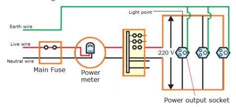
(b) The on/off switch of the mains is connected to the live wire.
