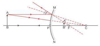
A concave mirror can form a magnified and virtual image. A convex mirror cannot form an enlarged image. When the object is placed between the pole and the focus of the mirror, the image formed is virtual, enlarged and erect.
