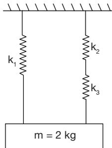
A mass of 2 kg is suspended by means of three springs as shown in figure. The spring constants  $k_1$ ,  $k_2$  and  $k_3$  are respectively 1 kN/m, 2 kN/m and 3 kN/m. The natural frequency of vibration of system is approximately (in rad/second)
