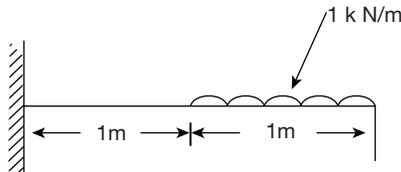
A cantilever beam of flexural rigidity  $5 \times 10^6 \text{ Nm}^2$  is loaded with a uniformly distributed load of 1 kN/m as shown in the figure. Deflection (in mm) at the free end of the beam is .
