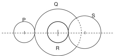
A compound gear train with gears  $P$ ,  $Q$ ,  $R$  and  $S$  has number of teeth 20, 40, 15 and 20 respectively. Gears  $Q$  and  $R$  are mounted on the same shaft as shown in the figure. The diameter of gear  $Q$  is twice that of gear  $R$ . If the module of the gear  $R$  is 4 mm, the centre distance (in mm) between the gears  $P$  and  $S$  is .
