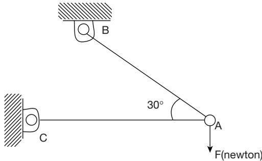
In the arrangement shown links  $AB$  and  $AC$  are uniform, made of same material, having same lengths and same areas of cross-section. When joint  $A$  is pulled down by a force  $F$  newton,  $|\Delta L_1|$  and  $|\Delta L_2|$  are the magnitudes of change in lengths of  $AB$  and  $AC$  respectively. Then,  $\frac{|\Delta L_1|}{|\Delta L_2|}$  is equal to.
