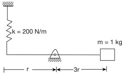
A thin uniform rod of mass 1 kg and length  $4r$  is hinged at a distance  $r$  from one end as shown in figure and held horizontally. A point mass of 1 kg is at right end and a light spring of stiffness  $k = 200$  N/m is at left end of rod. When the rod is slightly disturbed from its equilibrium position, it undergoes vertical angular oscillations with a frequency (in rad/s) equal to
