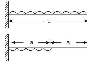
The loading is equivalent to a combination of downward and upward loadings as shown in figure.
