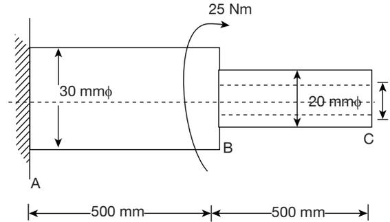
A stepped shaft  $ABC$ , fixed at  $A$  and hollow at portion  $BC$  is subjected to a twisting moment of  $25 \text{ Nm}$  at  $B$ . Shaft dimensions are as shown in the figure. Shear modulus  $G = 75 \text{ GPa}$ . The angle of twist at  $C$  (in degrees) is .
