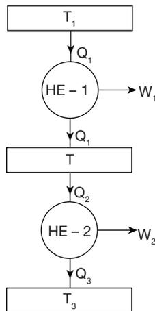
Two reversible heat engines  $HE-1$  and  $HE-2$  are connected in series and connected to thermal reservoirs at temperature  $T_1 = 1000$  K and  $T_3 = 300$  K as shown in figure. If the thermal efficiencies of the engines are same, the ratio of work done by the engines  $\left(\frac{W_1}{W_2}\right)$  is.
