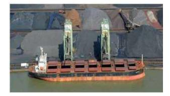
• Dry bulk refers to coal, iron ore, cement, and sand. They are not packaged separately, but transported in large quantities in the hold of a ship, wagon or lorry.
