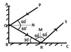
Ray PQ strikes the mirror AB at Q and gets reflected along QR according to the laws of reflection. The ray QR incident on mirror BC makes an angle of 30°
