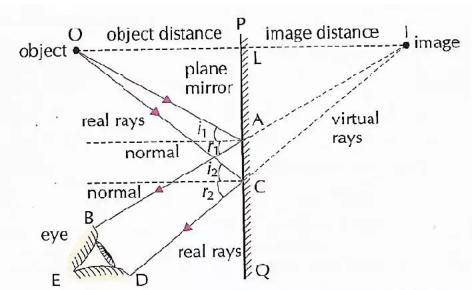
Characteristics of Image formed in plane mirror are:-1. Virtual Images are formed.2. Image formed is upright3. Object Distance is same as Image Distance4. Size of the Image formed is same as size of the object
