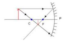
When an object is placed beyond the centre of curvature (C) of a concave mirror, the image is between the focus and centre of curvature, is real and inverted and is smaller than the object (or diminished).
