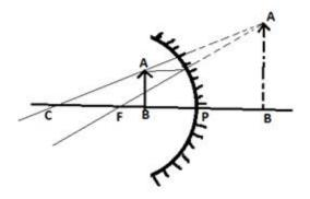
Converging mirror can be used to give an enlarged upright image of an object by placing the object between focus (F) and pole (P) of the concave mirror.
