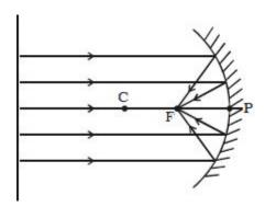
Since a concave mirror converges a parallel beam of light rays thus all the light rays parallel to the principal axis of a concave mirror, converge at the principal focus (F) after reflection from the mirror.
