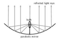
Bulb is placed at the focus of the torch reflector.
