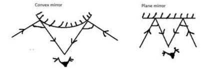
The images formed in the convex rear-view mirror will be smaller than those formed in the plane rear-view mirror.
