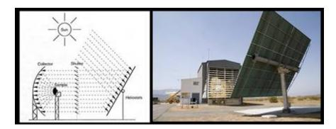
at the focus the solar furnace is placed of a large concave reflector.
