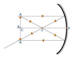
When an object is placed at the centre of curvature of a concave mirror, the image formed is at the centre of curvature, is real and inverted and is of same size as the object.
