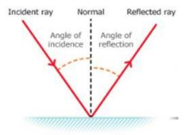
**First law of reflection:** The incidence ray, the reflected ray and the normal (at the point of incidence), all lie in the same plane.
