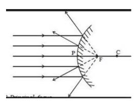
Since a convex mirror diverges a parallel beam of light rays thus all the light rays which are parallel to the principal axis of a convex mirror, appear to diverge from the principal focus (F) after reflection from the mirror.
