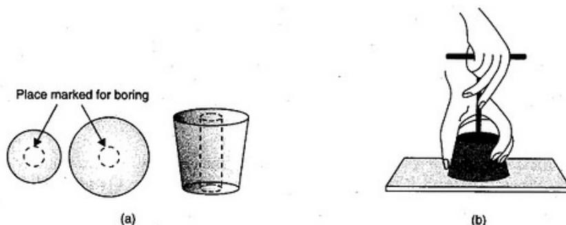
**Fig. 2.8.** (a) Marked cork, (b) Boring process.
