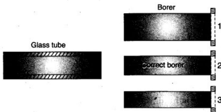
**Fig. 2.7.** Proper selection of the borer.
