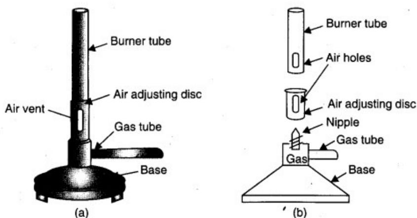
**Fig. 2.1.** (a) Bunsen burner, (b) Parts of Bunsen burner.
