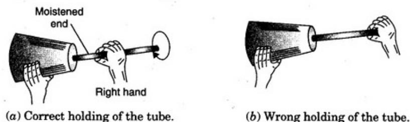
**Fig. 2.9.** Inserting the tube into the hole of the cork.
