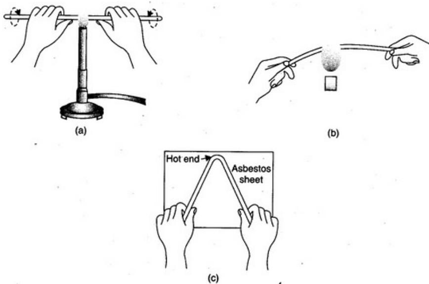
**Fig. 2.4.** (a) Heating the tube
