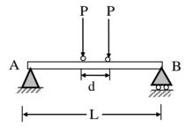
Each wheel transmits a load, P = 3kN and may occupy any position along the beam. If the beam is an I-section having section modulus,  $S = 16.2 \text{ cm}^3$ , the maximum bending stress (in GPa) due to the wheel loads is \_\_\_\_\_\_.
