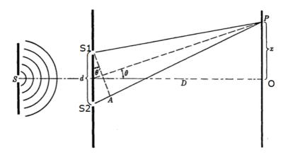
In Young's double slit experiment A monochromatic light is passed through a single narrow slit and falls on S1 and S2. These two slit acts as sources of light waves that interfere constructively and destructively at different points on the screen to produce a
