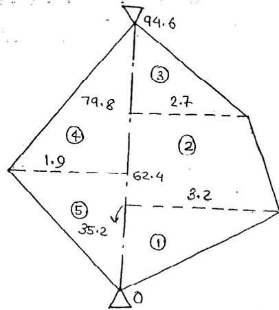
$$\begin{aligned} \text{Total area, } A &= A_1 + A_2 + A_3 + A_4 + A_5 \\ &= \underline{\underline{297.74 \text{ m}^2}} \end{aligned}$$
