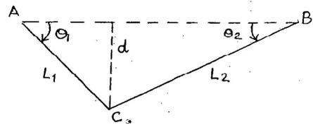
$$C_{MA} = L_1(1 - \cos \theta_1) + L_2(1 - \cos \theta_2) \quad \left\{ C_{MA} \text{ is always } -ve \right\}$$
