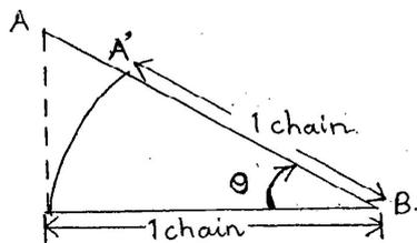
It is the correction to be applied in the field at every chain length and every point, where the slope changes.
