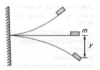
The load on the beam tends to displace it, say through a distance y. Restoring force will bring the beam to mean position and the beam starts vibrating.
