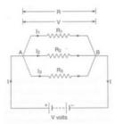
Suppose total current flowing in the circuit is I, then the current passing through resistance  $R_1$  will be  $I_1$ , current passing through resistance  $R_2$  will be  $I_2$  and current passing through resistance  $R_3$  will be  $I_3$ .
