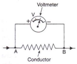
(e) Voltmeter has a high resistance so that it takes a negligible current from the circuit.
