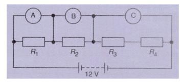
What would you expect the voltmeters A, B and C to read assuming that the connecting wires in the circuit have negligible resistance?
