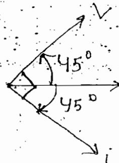
Ques:- Find circuit element for given voltage and current equations
