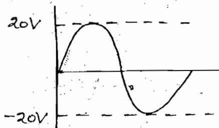
$$\text{Form factor} = \frac{V_{RMS}}{V_{av}}$$
