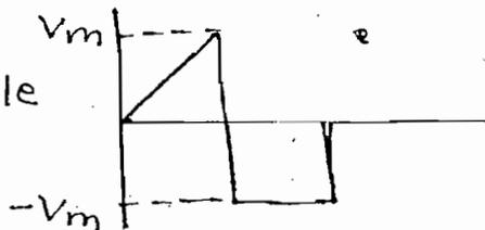
$$V_{av} = \frac{1}{2\pi} \left[ \int_0^{\pi} V dt + \int_{\pi}^{2\pi} V dt \right]$$
