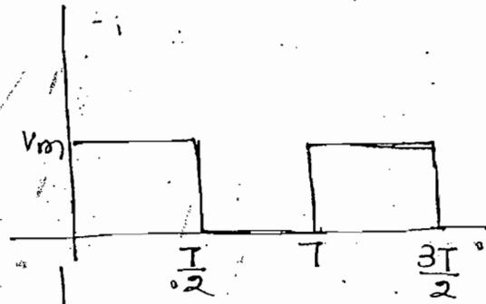
$$V_{RMS} = \sqrt{\frac{1}{T} \left[ \int_0^{T/2} V_m^2 dt + \int_{T/2}^T 0 dt \right]}$$
