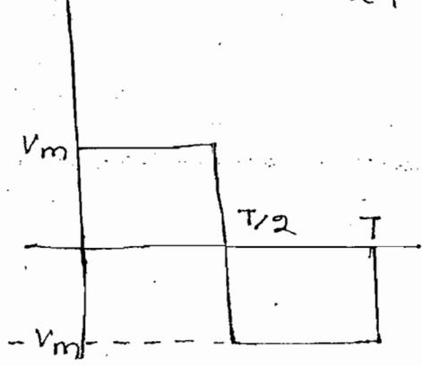
$$\rightarrow V_{RMS} = \sqrt{\frac{1}{T} \int_0^T v^2 dt}$$
