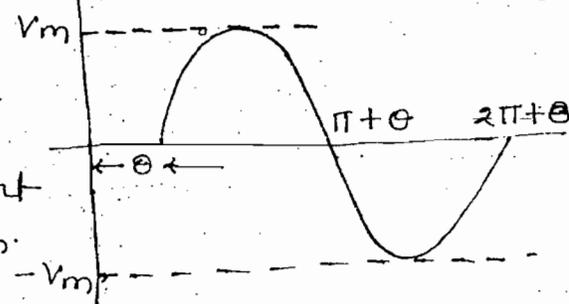
RMS value is independent on the <sup>position of</sup> starting of waveform. But it depends on the shape of waveform.
