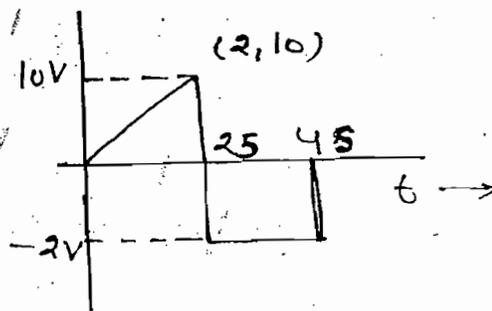
$$V_{RMS} = \sqrt{\frac{1}{4} \left[ \int_0^2 (5t)^2 dt + \int_2^4 (-2)^2 dt \right]}$$
