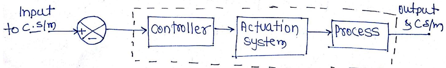
② Closed loop Control System:- In this case controller gets the information about the process variable as feedback is present.
