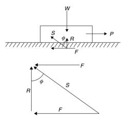
It is defined as the ratio of the limiting force of friction (*F*) to the normal reaction (*R*) between two bodies (see above figure, where a solid body rests on a horizontal plane). It is denoted by  $\mu$ .
