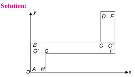
The x-axis and y-axis of reference are chosen as shown in the above figure such that the origin O coincides with the point A of the figure and the axes coincide with the left most and bottom most lines of the figure respectively. The position of the centre of gravity is determined with respect to the origin O.
