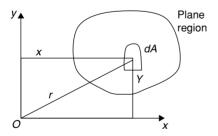
The moment of inertia of the area about the *x*-axis and *y*-axis respectively are:
