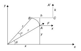
To illustrate the principle of work, let us consider a body at equilibrium at a point A. A force F acts on the body and displaces it to the point A', where the displacement consists of the following:
