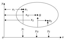
The above figure shows an irregular lamina of total area A whose center of gravity is to be determined. Let the lamina be composed of small areas  $a_1, a_2 \dots$  etc. Such that:
