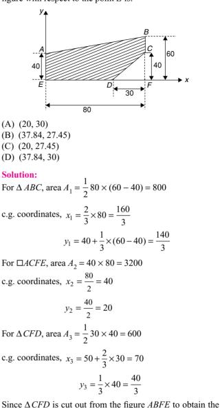
hatched figure, the area of  $\Delta CFD$  is assigned a negative sign.
