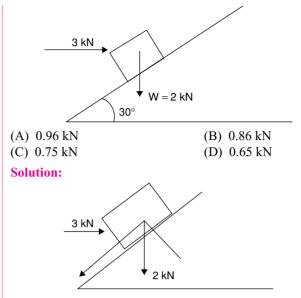
Applying the conditions of equilibrium and summing the force parallel and perpendicular to the plane, we have:
