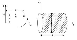
For example, in the above figure, the curved surface of a cylinder is obtained by rotating the line *AB* about the *x*-axis.
