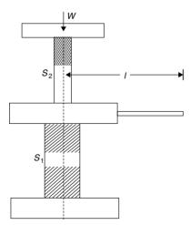
This spindle carries both internal as well as external threads. The spindle  $S_2$  is engaged to spindle  $S_1$  by means of an internal thread. When spindle  $S_1$  ascends, the spindle  $S_2$  descends. This is also known as 'Differential Screw' jack. The principle of working of this jack is similar to the one as described in the above figure.
