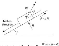
For motion down the plane,  $P = \frac{m \sin(\alpha - \phi)}{\cos(\theta + \phi)}$
