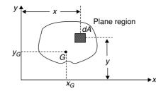
Let dA be a differential (i.e., infinitesimal) area located at the point (x, y) in the plane region area A.
