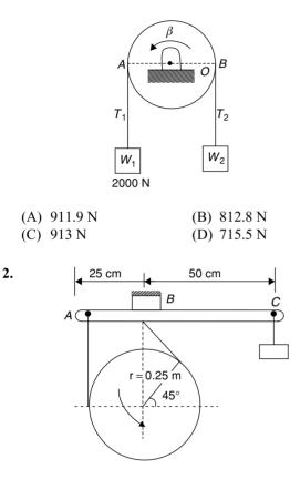
A rotating wheel is braked by a belt *AB* attached to the lever *ABC* hinged at *B*. The coefficient of friction between the belt and the wheel is 0.5. The braking moment exerted by the vertical weight W = 200 N is:
