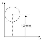
If the density of the material making up the circular crosssection is  $7800 \text{ kg/m}^3$ , the weight of the ring generated is: (A) 82.6 N (B) 94.4 N
