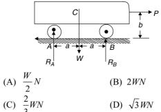
**Direction for question 5:** When it is pulling a wagon, the draw bar pull *P* is just equal to the total friction at the points of contact, *A* and *B*.
