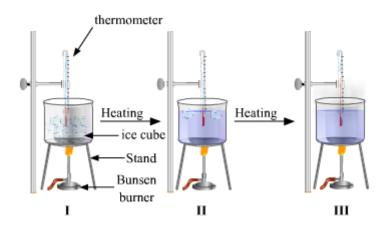
**Result**: In the beginning, the temperature of ice is below 0°C. When ice begins melting, the temperature is recorded to be 0°C. Temperature remains constant at 0°C untill all the ice melts. The continued heating of water causes its temperature to rise.
