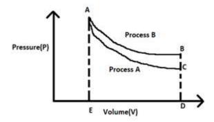
From this diagram, we can see that that area under the curve of process A(ACDE) which represents the adiabatic process with greater slope is less than that of the area under the curve of process B(ABDE), which represents the isotherm.
