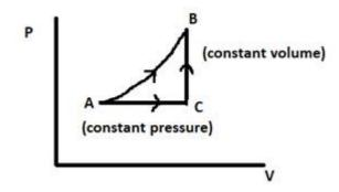
We consider the process AB to be composed of two processes, AC(at constant pressure) and CB(at constant volume), such that AB = AC + CB. C is the molar heat capacity of AB,  $C_p$  is the molar heat capacity of AC(constant pressure) and Cv is the molar heat capacity of CB(constant volume).
