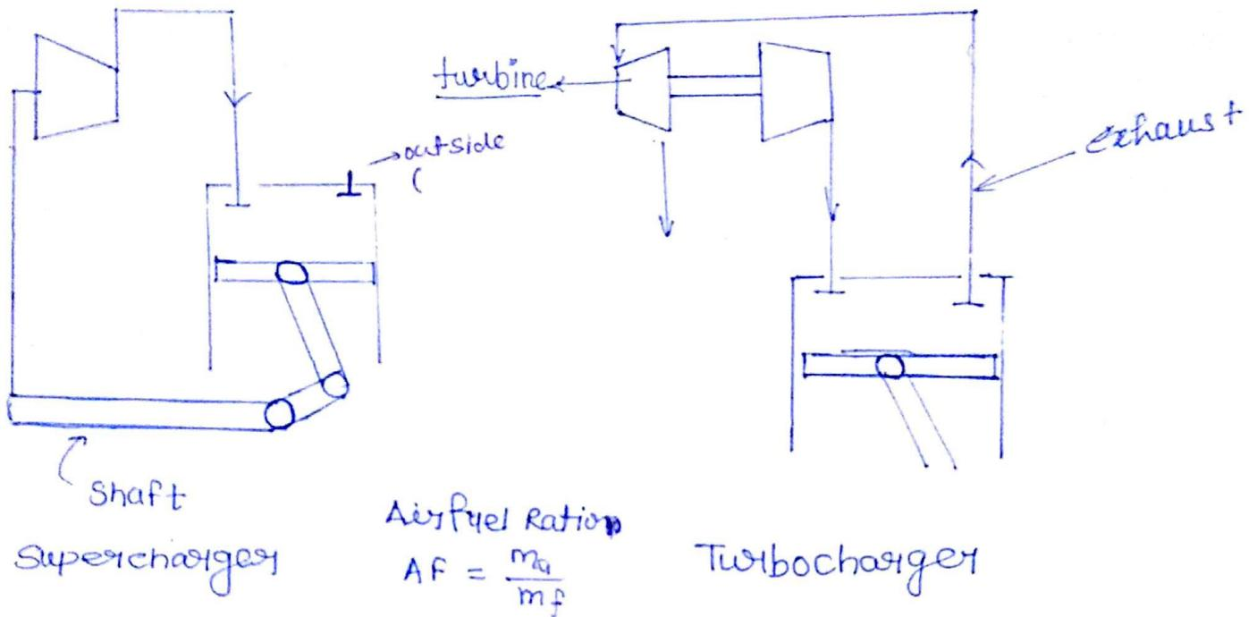
Supercharger is a rotary compressor it attached before the cylinder in diesel engine and before the carburetor in petrol engine. On using a supercharger, the mass of air circulator is more. The final pressure after super charging is 1.5 times to 2 times the entry pressure.
