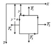
NOTE : Now as loop goes down, magnetic flux linked with it increases, hence induced current flows in such a direction so as to reduce the magnetic flux linked with it. Hence, induced current flows in anticlockwise direction.
