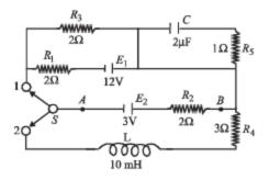
(a) The switch S is in position '1'. Find the poten tial difference  $V_A - V_B$  and the rate of production of joule heat in  $R_1$ .
