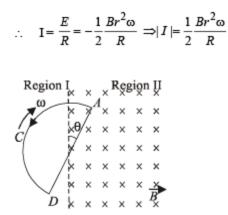
(ii) The loop is entering in the magnetic field and hence magnetic lines of force passing through the loop is increasing in the downward direction. Therefore, current will flow in the loop in such a direction which will oppose the change. The current will flow in the anticlockwise direction.
