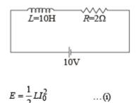
This is the maximum energy stored in the inductor. The current in the circuit for one fourth of this energy can be found as
