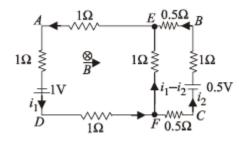
NOTE : As the magnetic field increases in the downward direction, an induced emf will be produced in the AEFD as well as in the circuit EBCF such that the current flowing in the loop creates magnetic lines of force in the upward direction (to the plane of paper).
