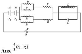
Solution. NOTE : After a long time capacitor will be fully charged, hence no current will flow through capacitor and all the current will flow from inductor. Since current is D.C., resistance of L is zero.
