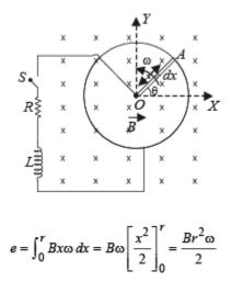
(b) The above diagram can be reconstructed as the adjacent figure. e is a constant. O will accumulate positive charge and A negative. When the switch S is closed, transient current at any time t, when current I is flowing in the circuit,
