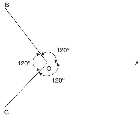
At a stressed point in a two dimensional stress system, strain were measured to 3 directions OA, OB and OC,  $120^\circ$  to each other. The observed strains are  $e_A = 300 \times 10^{-6}$ ,  $e_B = -225 \times 10^{-6}$  and  $e_C = 100 \times 10^{-6}$ . Value of strain at an angle  $90^\circ$  clockwise to OA (in micron) is \_\_\_\_\_.
