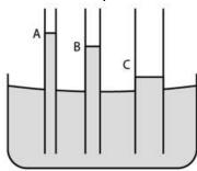
Surface tension of water = T =  $7.5 \times 10^{-2} \text{ N/m}$ Considering cos  $\theta$  = 1 Radius of capillary A =  $r_A$  = 0.5 mm =  $0.5 \times 10^{-3}$  m
