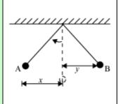
You will find that the distance y < x. This is because air particles present in the medium oppose the motion of the pendulum. Hence, its distance decreases continuously until the bob comes to rest.
