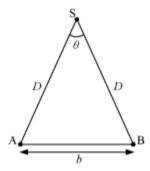
Far-away object (S) is observed from two different positions (A and B).
