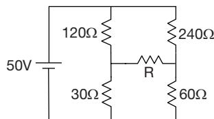
What is the power delivered to resistor  $R$  in the above circuit?
