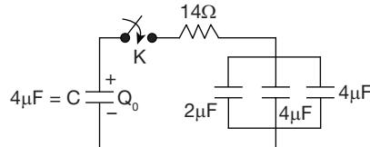
34. Determine the voltage drop across resistor at  $t < T$  where  $T$  is time constant.
