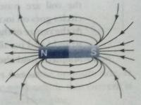
8. Put the compass at some other points near the N-pole of the magnet and draw another magnetic field lines. Similarly, draw many field lines on both the sides of the bar magnet as shown in figure.
