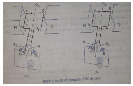
The current generated by such a simple dynamo is uni-directional. As long as the coil is rotating, the direct current flows through the device connected to the terminals of the generator.
