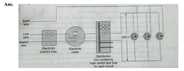
A fuse in a circuit prevents damage to the appliances and the circuit due to overloading. Otherwise, the appliances or the circuit may be damaged.
