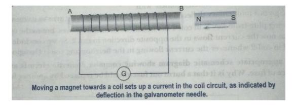
(b) Connect the ends of the coil to a galvanometer
