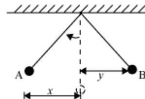
You will find that the distance  $y < x$ . This is because air particles present in the medium oppose the motion of the pendulum. Hence, its distance decreases continuously until the bob comes to rest.
