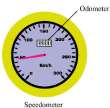
Modern vehicles use **speedometers** that measure speed in units of km/h. They also include **odometers** that record the total distance travelled by vehicles in units of kilometre (km). A simple speedometer with an odometer is shown in the given figure.
