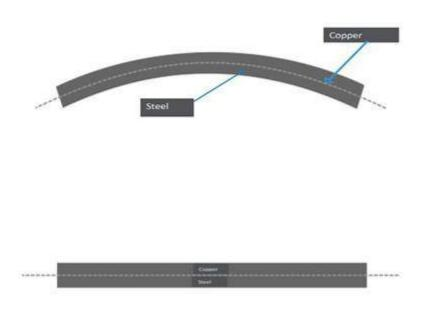
Linear expansion coefficient of copper is greater than the steel ( $\alpha_{copper} > \alpha_{steel}$ ). So, on heating copper gets more expansion than steel. So the bimetallic strip will bend with the copper on the convex side.
