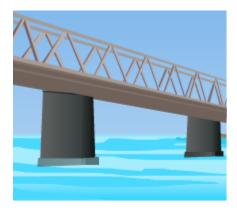
You will notice that this bridge has several irons beams arranged triangularly between horizontal parallel beams on either side. The triangles formed between the parallel beams are all of the same area. Such an arrangement ensures that the load of traffic does not result in bridge failure. The use of the triangular shape for this purpose is because this shape does not deform easily. This shape is unlike, say, the rectangular shape which can deform easily under force.
