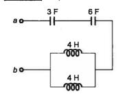
**Q.23** For the circuit shown below resonant frequency  $f_0$  is \_\_\_\_\_ kHz.
