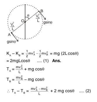
from equation (1) and (2)  $T_A - T_B = 6 \text{ mg } \cos\theta$  Ans. The component of accelerations of ball at A and B are as shown in figure.
