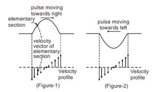
When both the pulses completely overlaps, the velocity profiles of both the pulses in overlap region are identical. By superposition, velocity of each elementary section doubles. Therefore K.E. of each section becomes four times. Hence the K.E. in the complete width of overlap becomes four times, i.e., 4k.
