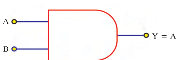
Figure 7.48 Symbol of AND Gate
