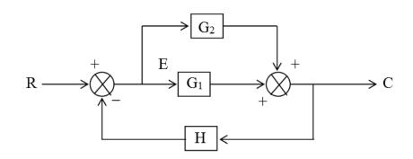
**Q.2** The number of forward paths and the number of non-touching loop pairs for the signal flow graph given in the figure are, respectively,
