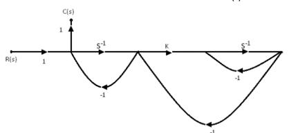
**Q.4** Three blocks  $G_1$ ,  $G_2$  &  $G_3$  are connected in some fashion such that overall transfer function is  $\frac{G_1+G_3(1+G_1G_2)}{1+G_1G_2}$ . The blocks are connected in the following manner
