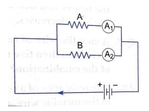
**Ans.** Ammeter  $A_2$  shows higher reading. Since wire  $A_1$  is longer, it has greater resistance and so draws lesser current. So more current. So more current flows through B and  $A_2$  shows higher reading.
