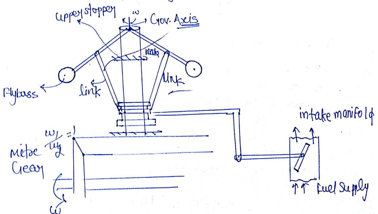
$\Rightarrow$  load  $\downarrow \Rightarrow$  speed  $\uparrow \Rightarrow$  sleeve will move upward
