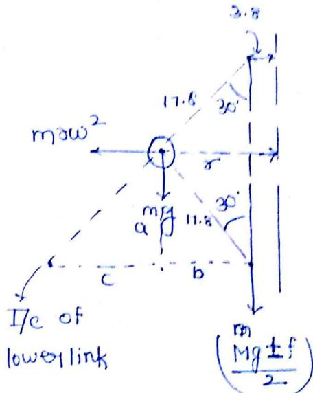
$$m\omega^2 a = mg c + \left(\frac{Mg + f}{2}\right)\left(\frac{b}{a} + c\right)$$
