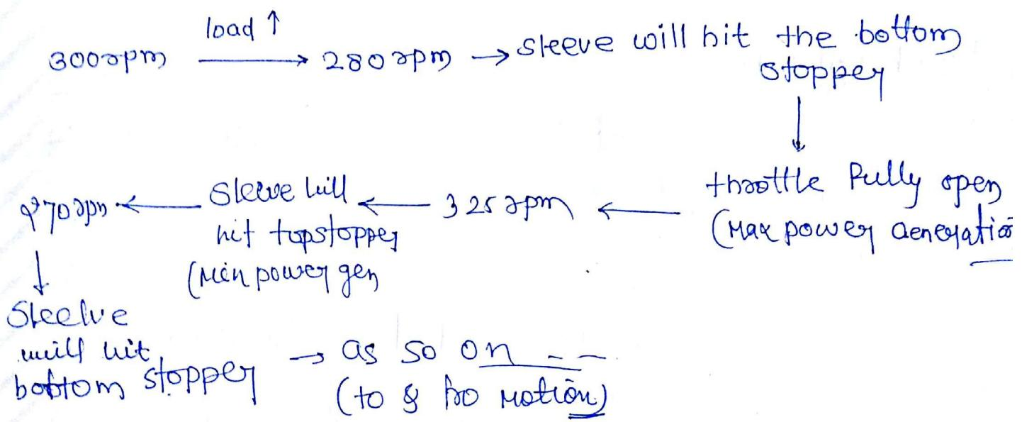
It is an excessively fast to and fro motion of the sleeve between the stoppers as a result a big noise, vibrations as well as the fluctuation of speed will be introduce in the system and of few moments stoppers will be out of order and the system will be out of control of governor.
